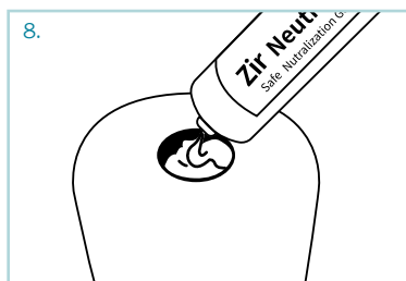
8. Apply Zir Neutralization Gel to the top of the Safe Shell(1) to close the injection port.
